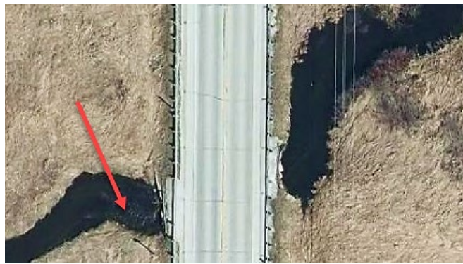
Figure 12.2 Scour hole at the downstream end of undersized culvert in Waushara County
