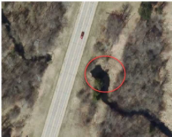
Figure 12.4 Downstream scour holes suggest high velocities at culvert outfalls.
