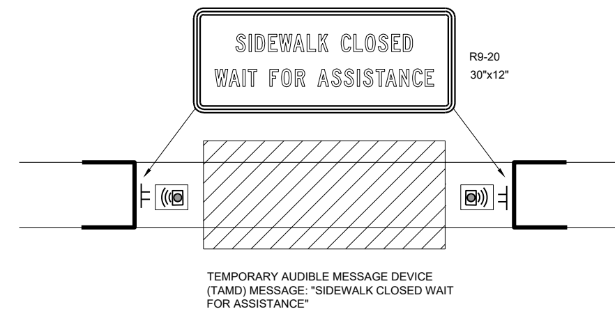
TEMPORARY PEDESTRIAN FLAGGING
