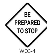
USE OF WO3-4 SIGN IS OPTIONAL. WHEN USED, THIS SIGN SHALL BE LOCATED BETWEEN THE W20-7A AND W20-4A SIGNS, USING SPACING "A".
