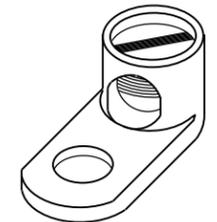
**TYPICAL MECHANICAL CONNECTOR LUG**
