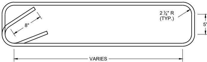
END ANCHOR STIRRUP BAR BENDING DETAIL
