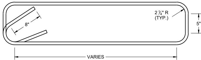
END ANCHOR STIRRUP BAR BENDING DETAIL
