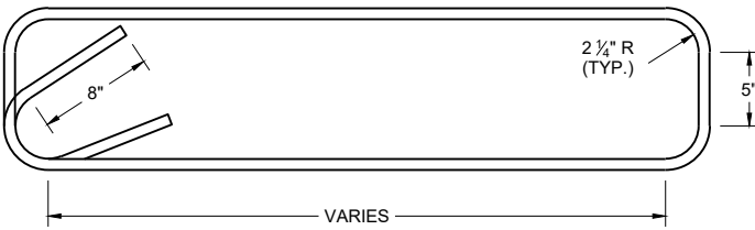
END ANCHOR STIRRUP BAR BENDING DETAIL
