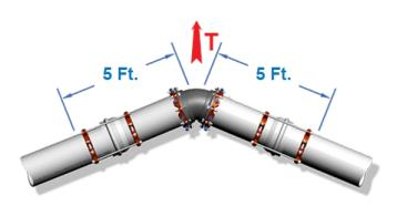
\*all joints within the calculated length must be restrained
