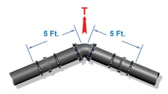
\*all joints within the calculated length must be restrained
