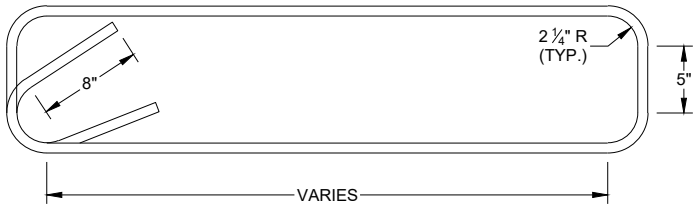
END ANCHOR STIRRUP BAR BENDING DETAIL
