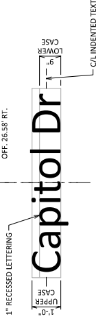
ROAD NAME PANEL DETAILS - SOUTH PARAPET
