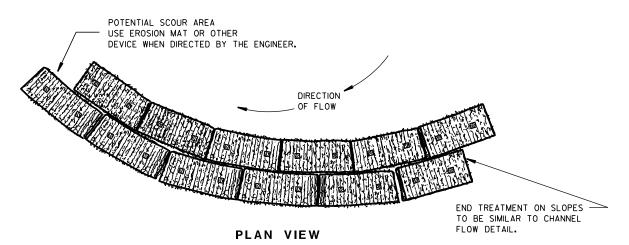
WHEN ALTERING THE DIRECTION OF FLOW
