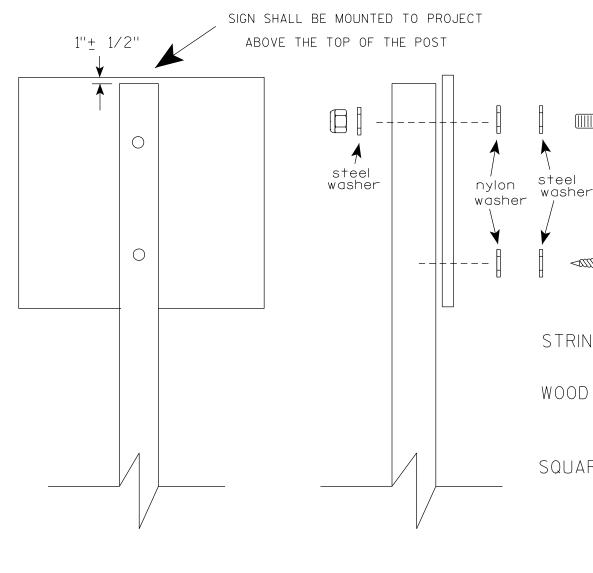
Nuts, bolts and lags used for mounting signs shall have hexagonal heads and shall be either:
