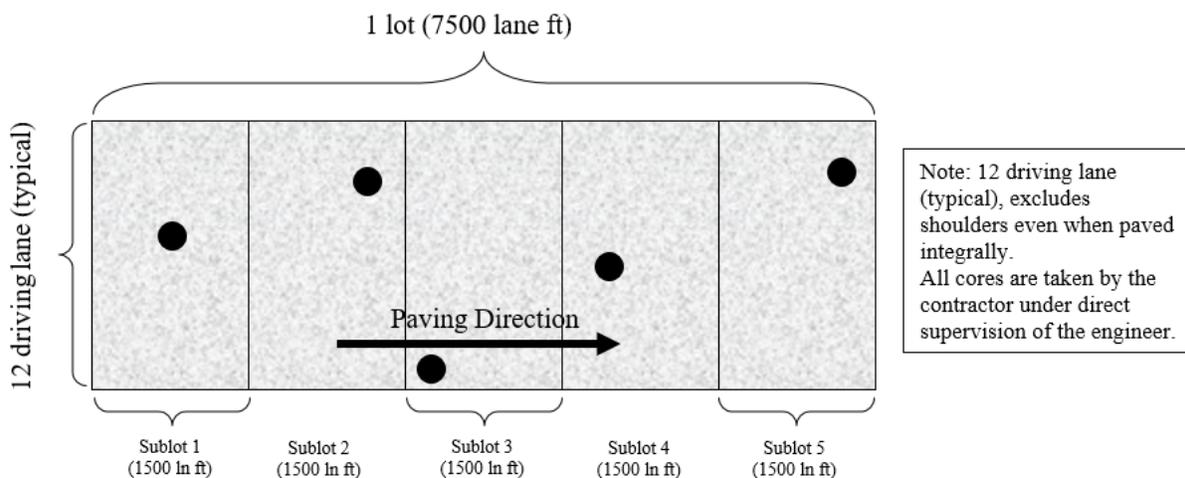
**Figure 5: Example core density locations for traffic lanes**
