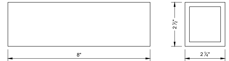
FOUNDATION TUBE - ANCHOR CABLE TUBE (QQ2)
