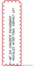
NOTE: CONCRETE ENCASUREMENT SHALL ONLY BE USED IN AREAS WHERE COVER IS TO BE FLUSH WITH PAVEMENT OR CONCRETE. CONCRETE ENCASUREMENT SHALL NOT BE USED IN NON-TRAFFIC AREAS.
