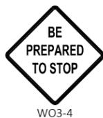
USE OF W03-4 SIGN IS OPTIONAL. WHEN USED, THIS SIGN SHALL BE LOCATED BETWEEN THE W20-7A AND W20-4A SIGNS, USING SPACING "A".
