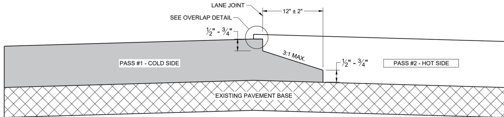
**TYPICAL PAVEMENT CROSS SECTION
