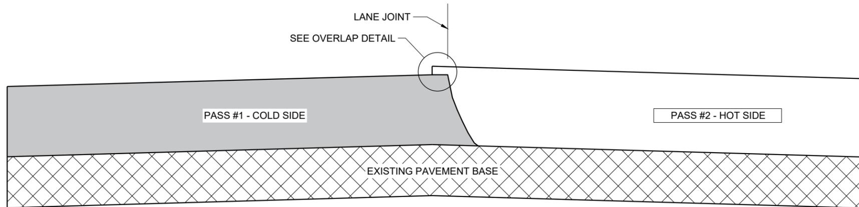
**TYPICAL PAVEMENT CROSS SECTION
