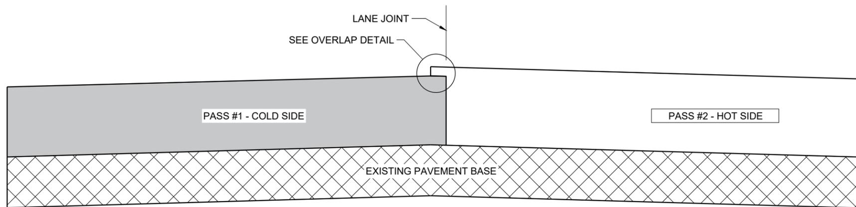
**TYPICAL PAVEMENT CROSS SECTION
