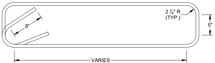
END ANCHOR STIRRUP BAR BENDING DETAIL
