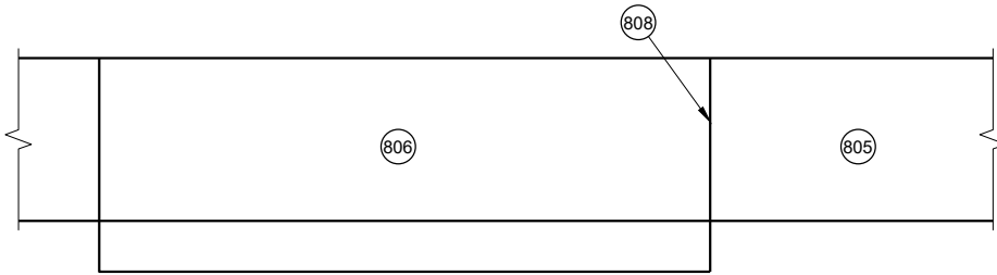
CONCRETE BARRIER EXTENSION NEAR END ANCHORAGE
