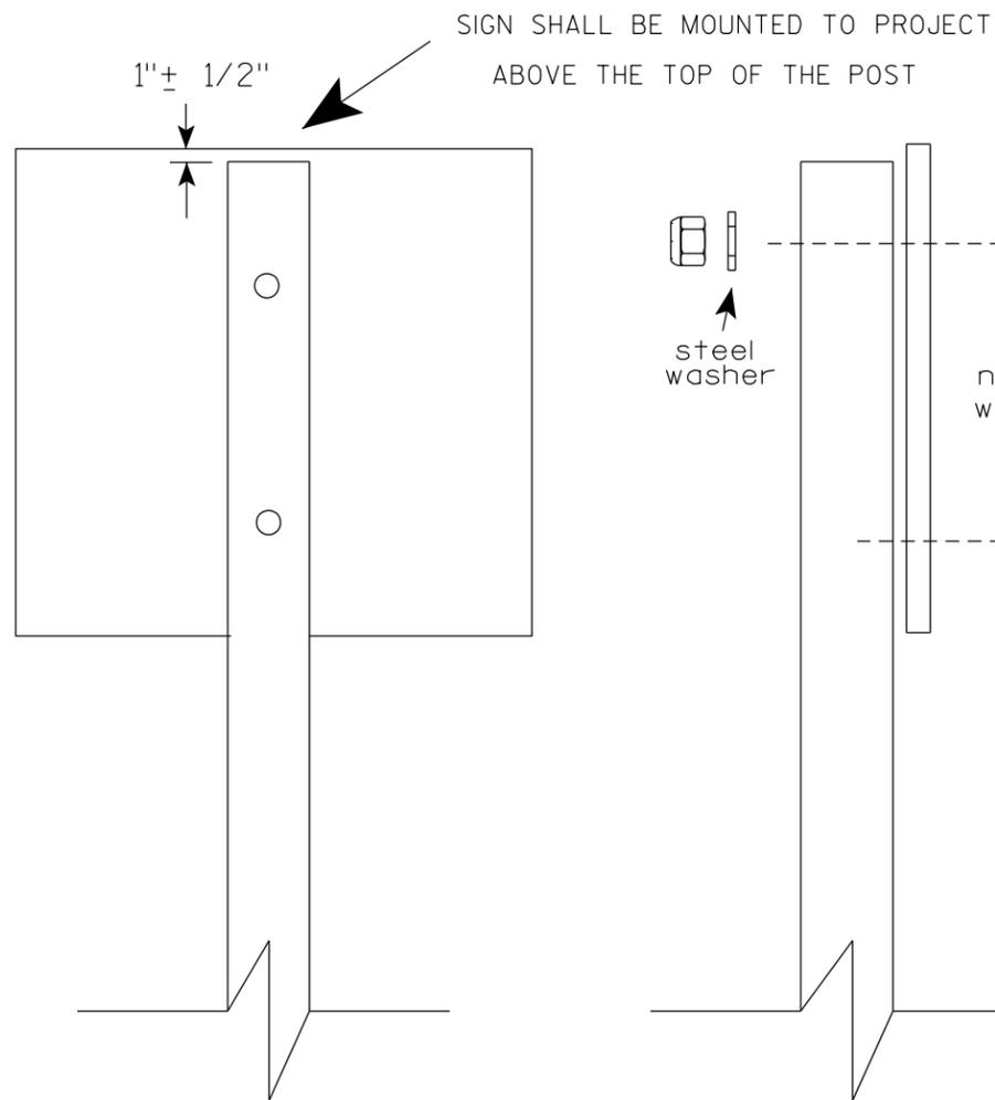
Nuts, bolts and lags used for mounting signs shall have hexagonal heads and shall be either :
