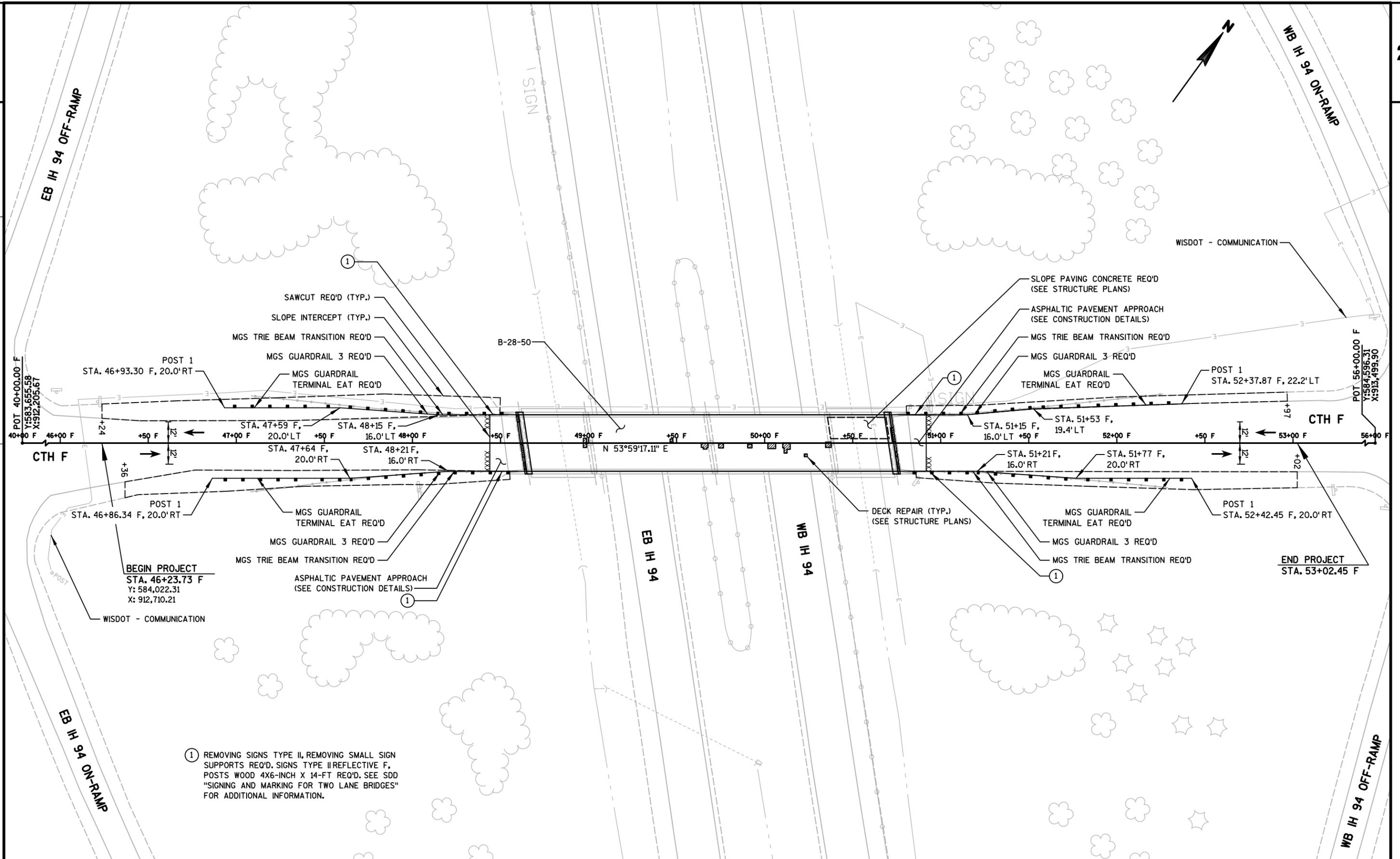
① REMOVING SIGNS TYPE II, REMOVING SMALL SIGN SUPPORTS REQ'D, SIGNS TYPE II REFLECTIVE F, POSTS WOOD 4X6-INCH X 14-FT REQ'D. SEE SDD "SIGNING AND MARKING FOR TWO LANE BRIDGES" FOR ADDITIONAL INFORMATION.
