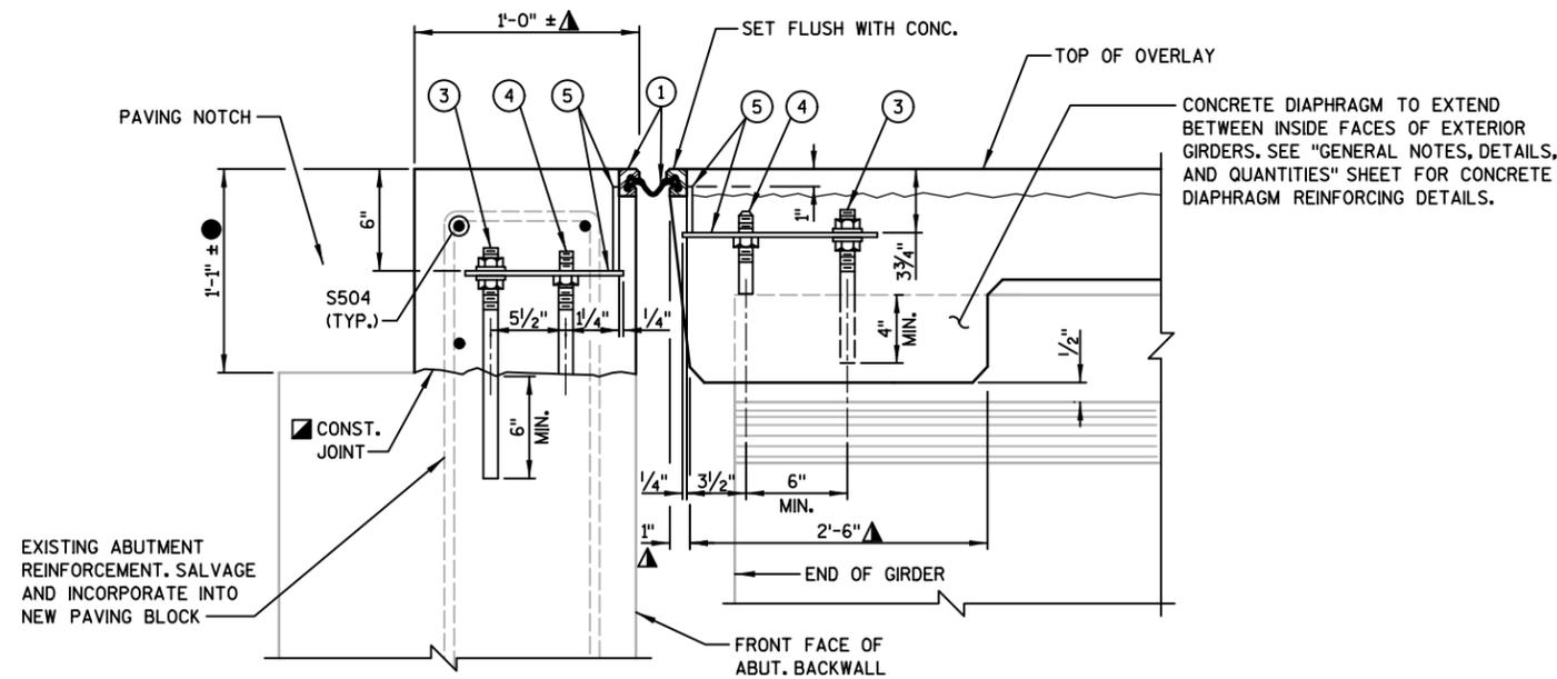
**SECTION THRU JOINT AT ABUTMENT**
