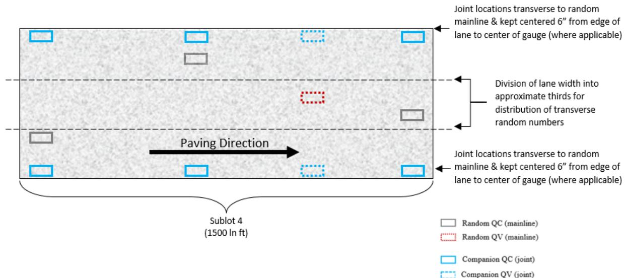
**Further Explanation of PAY ADJUSTMENT FOR HMA PAVEMENT LONGITUDINAL JOINT DENSITY
