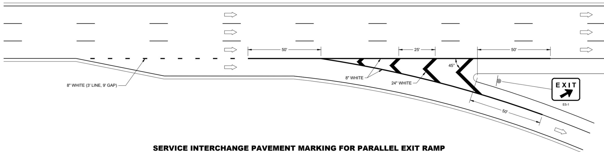
**SERVICE INTERCHANGE PAVEMENT MARKING FOR PARALLEL EXIT RAMP**
