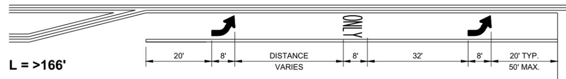
\*(SEE TURN LANE OPTIONS FOR PLACEMENT OF PAVEMENT MARKING ARROWS AND WORDS)
