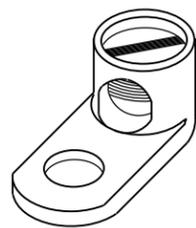
**TYPICAL MECHANICAL CONNECTOR LUG**
