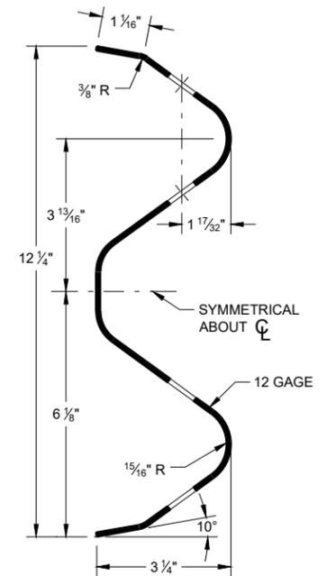
**SECTION THRU W-BEAM RAIL**
