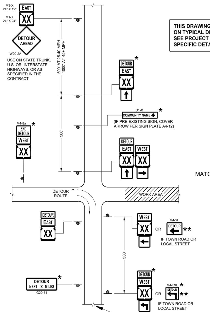
THIS DRAWING PROVIDES GENERAL GUIDANCE ON TYPICAL DETOUR SIGN LAYOUT AND SPACING. SEE PROJECT DETOUR SIGNING SHEETS FOR SPECIFIC DETAILS FOR EACH PROJECT.
