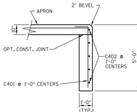
**SECTION THRU OUTLET CUT OFF WALL**
