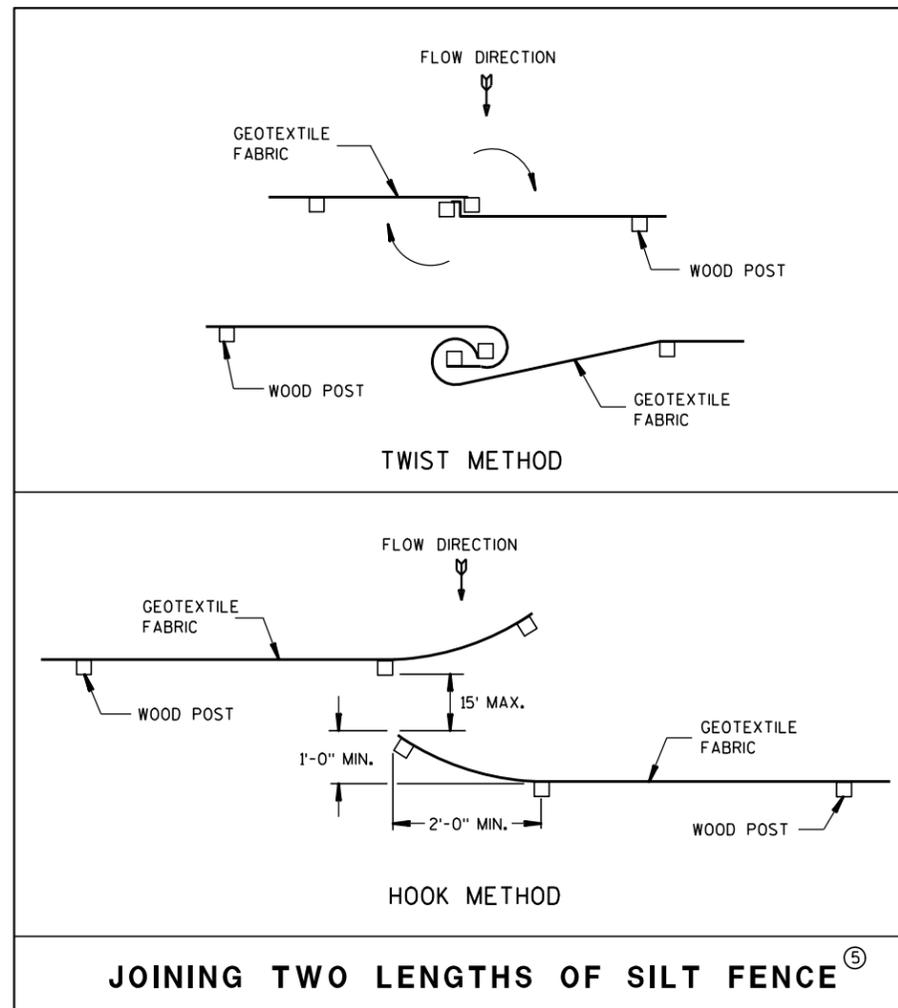
JOINING TWO LENGTHS OF SILT FENCE ⑤
