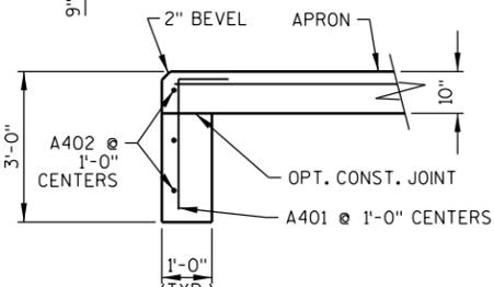
**SECTION THRU INLET CUT OFF WALL
