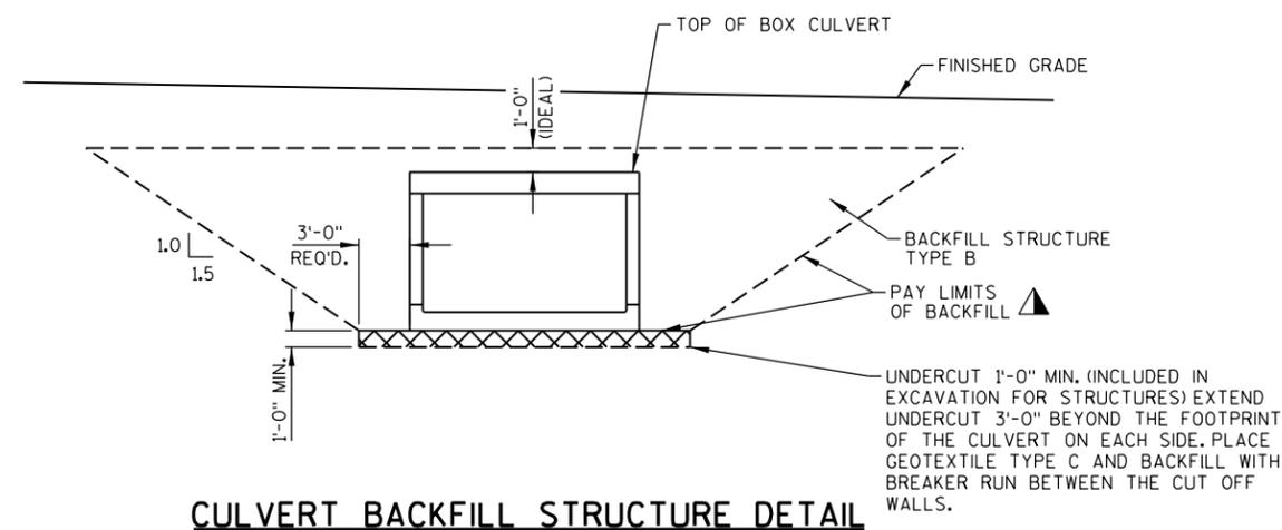
CULVERT BACKFILL STRUCTURE DETAIL
