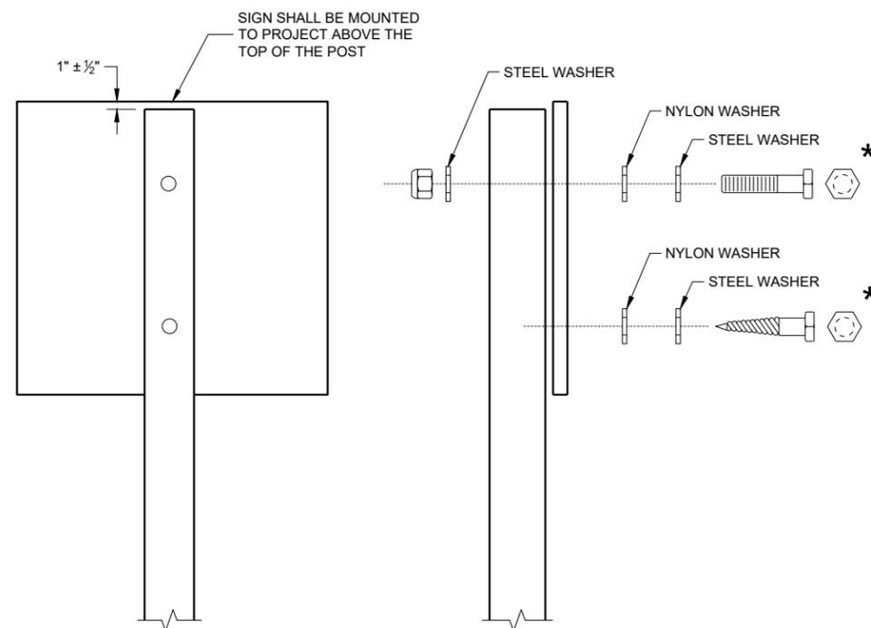
NUTS, BOLTS AND LAGS USED FOR MOUNTING SIGNS SHALL HAVE HEXAGONAL HEADS AND SHALL BE EITHER:
