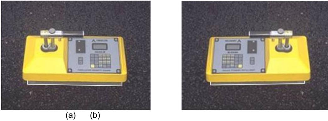
**Figure 2: Nuclear gauge orientation for (a) 1<sup>st</sup> one-minute reading and (b) 2<sup>nd</sup> one-minute reading**
