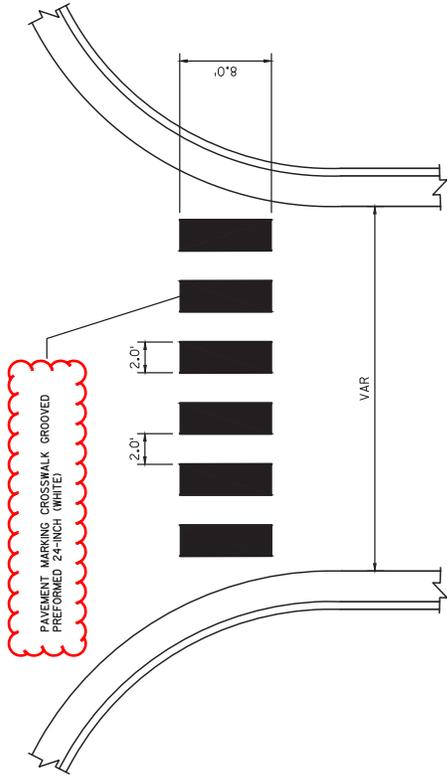
PAVEMENT MARKING CROSSWALK DETAIL
