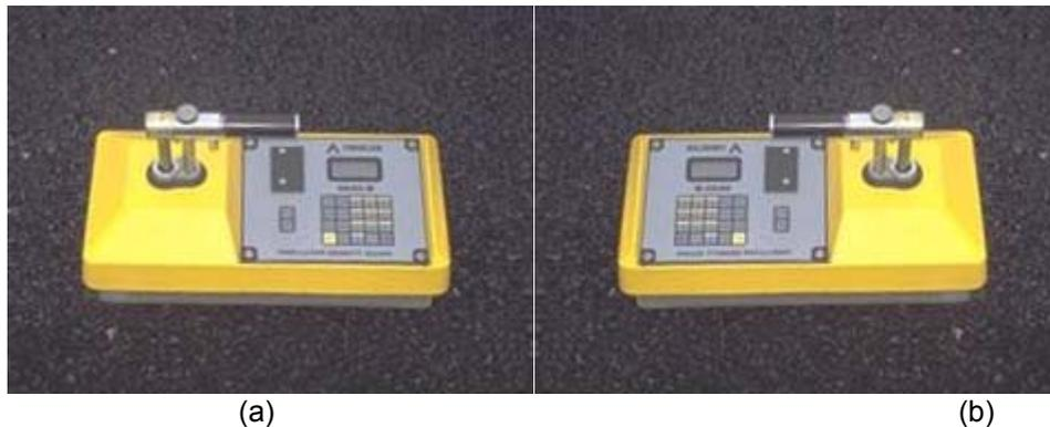
**Figure 2: Nuclear gauge orientation for (a) 1<sup>st</sup> one-minute reading and (b) 2<sup>nd</sup> one-minute reading**
