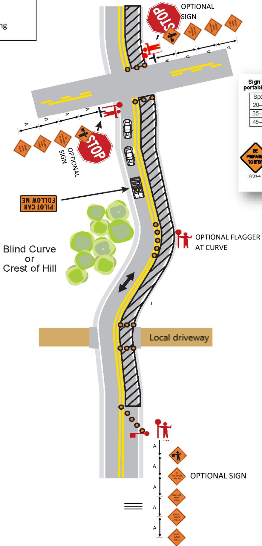
**Sign spacing and temporary portable rumble strip placement**
