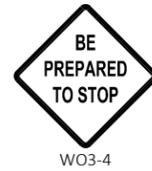
USE OF W03-4 SIGN IS OPTIONAL. WHEN USED, THIS SIGN SHALL BE LOCATED BETWEEN THE W20-7A AND W20-4A SIGNS, USING SPACING "A".
