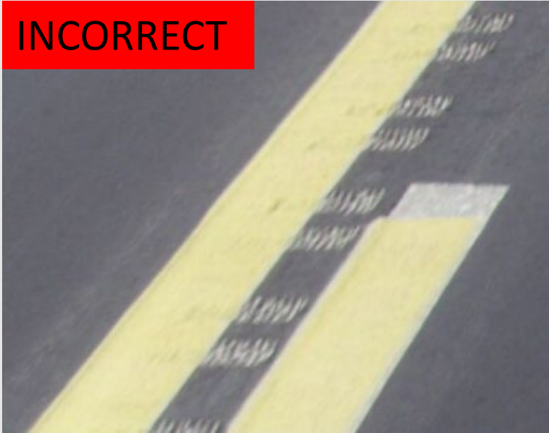
To narrow for wet reflective epoxy
