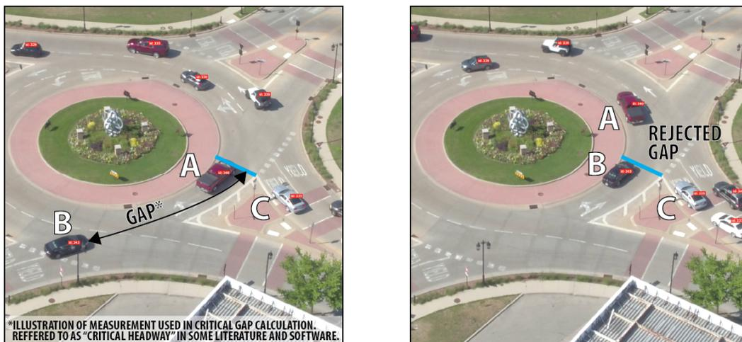
In the case illustrated in [Figure 2](#), vehicle C rejected the gap between vehicles A and B because vehicle C did not enter the roundabout during the gap. If vehicle C would have entered the gap, the length of time between vehicles A and B crossing the conflicting line would have been vehicles C's accepted gap.
