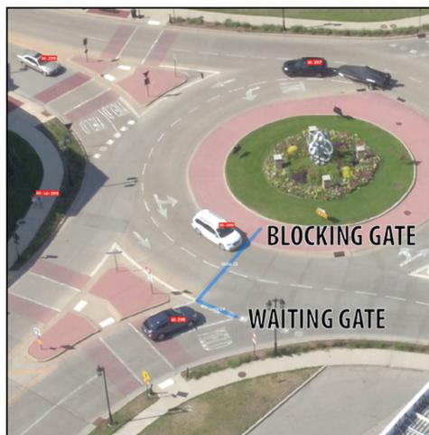
The DataFromSky Viewer software detects when a vehicle is stopped at the waiting gate and then detects when circulating vehicles cross the blocking gate. The software outputs the length in
