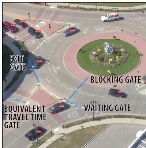
The equivalent travel time gate was placed at a location where the travel time between the exit gate and the equivalent travel time gate was approximately equal to the equivalent travel time, as shown in [Figure 15](#) in Section 3.2.1. The equivalent travel time was added to the gap time in accordance to the equation in [Figure 16](#) in Section 3.2.1 for critical gap estimates taking adjacent exiting vehicles into consideration.
