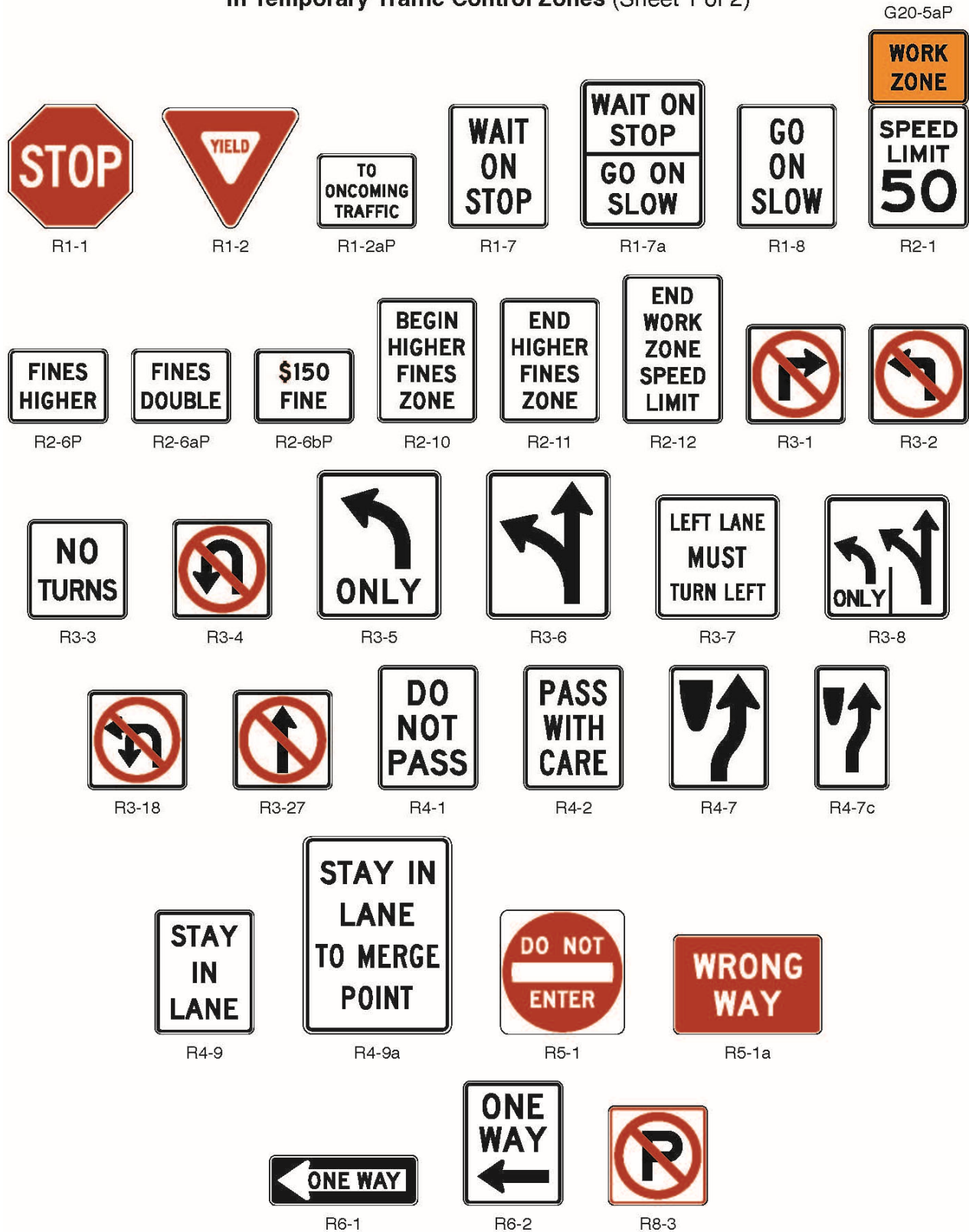
Figure 6G-1. Regulatory Signs and Plaques in Temporary Traffic Control Zones (Sheet 1 of 2)
