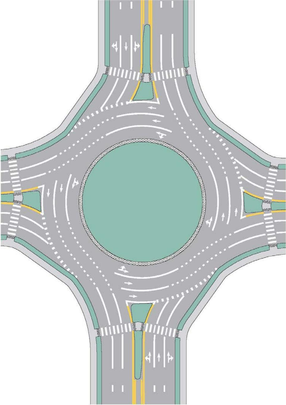
Figure 3C-12. Example of Markings for a Three-Lane Roundabout with Two-Lane Exits
