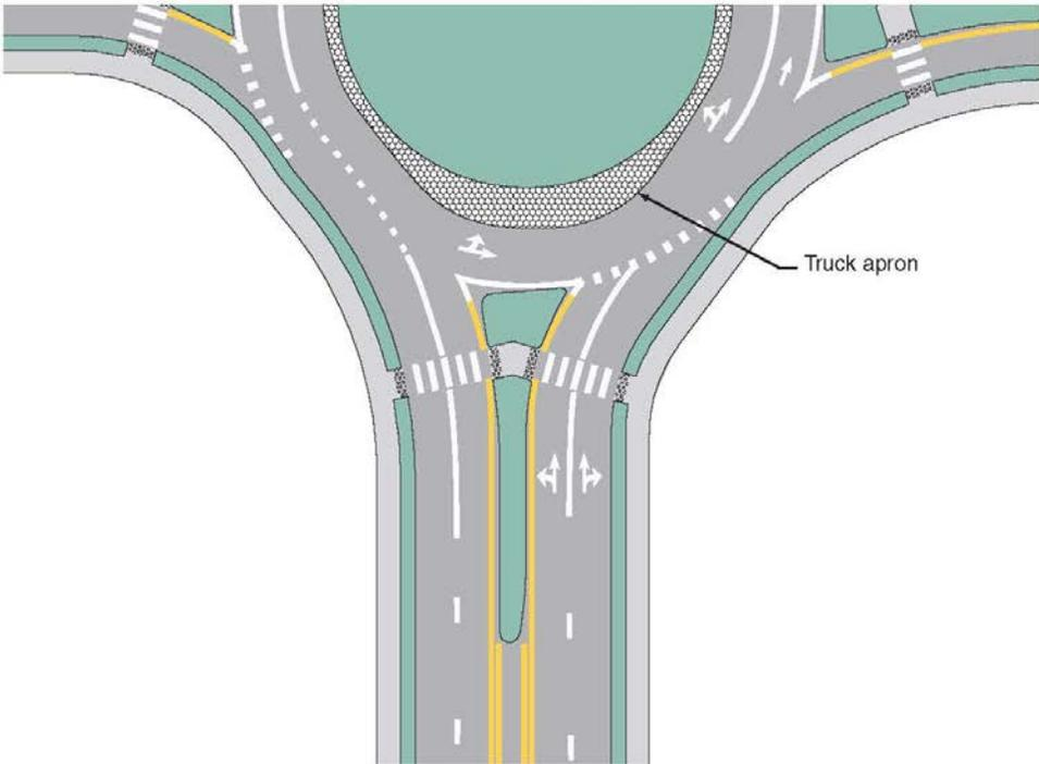
Figure 3C-5. Example of Markings for a Two-Lane Roundabout with One-Lane Exits
