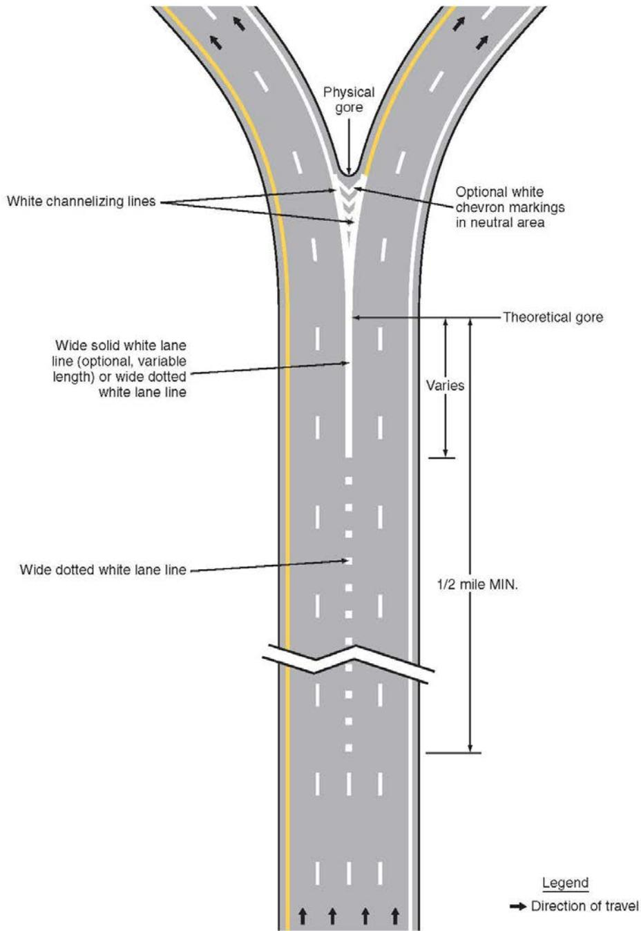
**Figure 3B-10. Examples of Applications of Freeway and Expressway Lane-Drop Markings (Sheet 5 of 5)**
