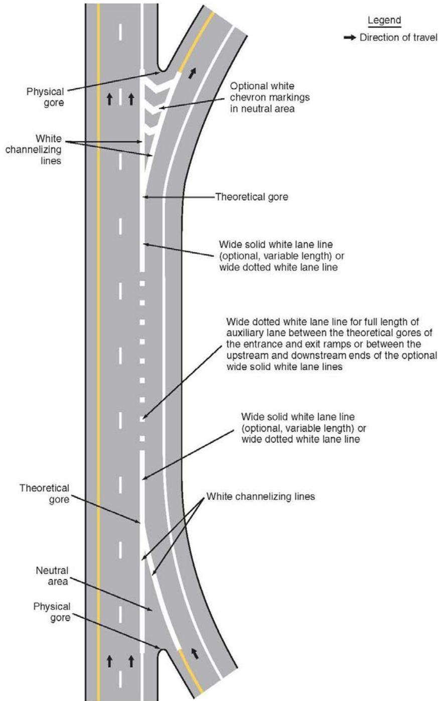
Figure 3B-11. Examples of Applications of Conventional Road Lane-Drop Markings
