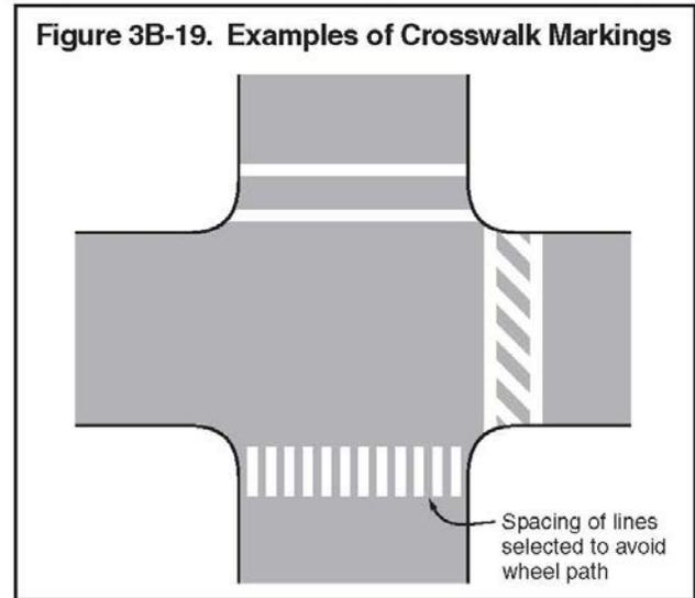
15 If used, the diagonal or longitudinal lines should be 12 to 24 inches wide and separated by gaps of 12 to 60 inches. The design of the lines and gaps should avoid the wheel paths if possible, and the gap between the lines should not exceed 2.5 times the width of the diagonal or longitudinal lines.
