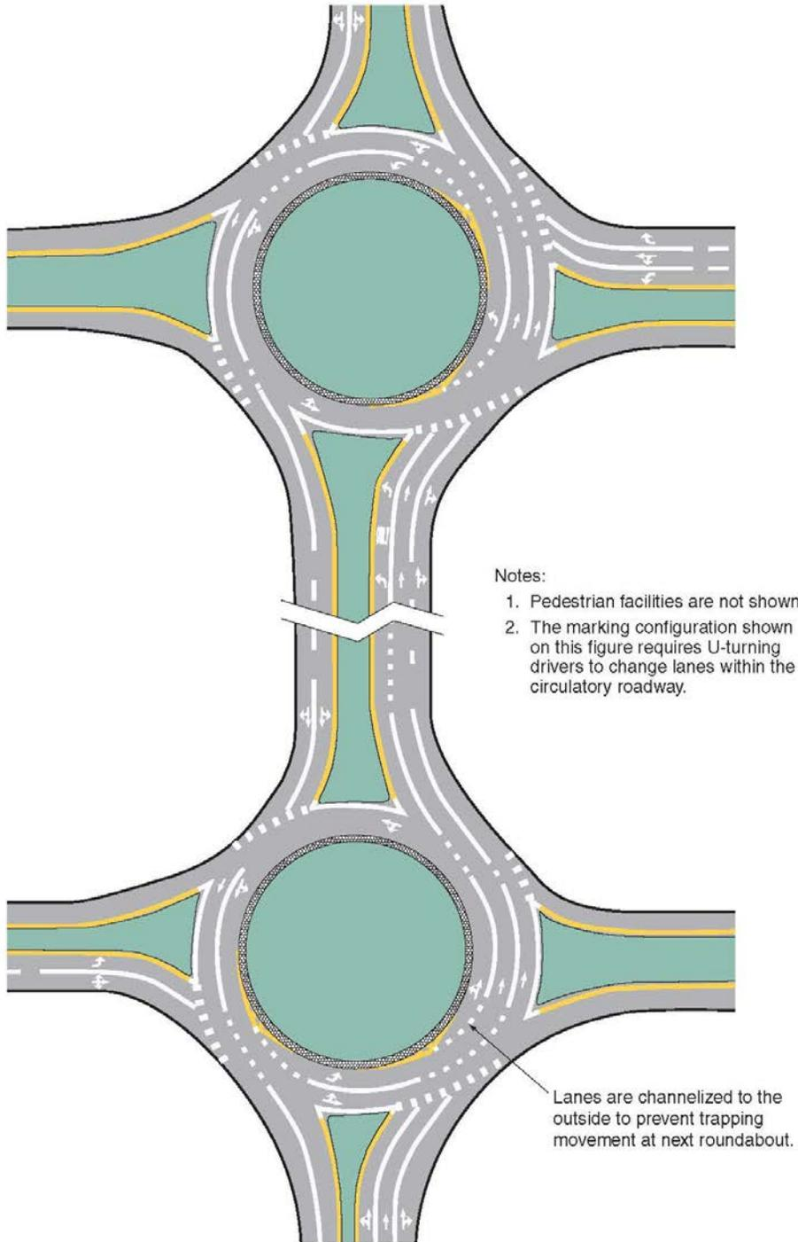
**Figure 3C-14. Example of Markings for a Diamond Interchange with Two Circular-Shaped Roundabout Ramp Terminals**
