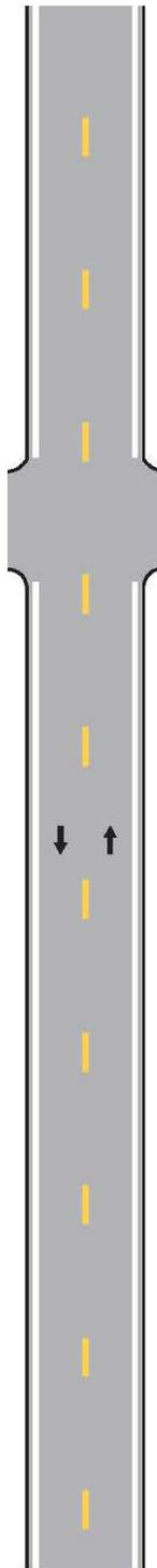
B - Typical two-lane, two-way marking with no-passing zones
