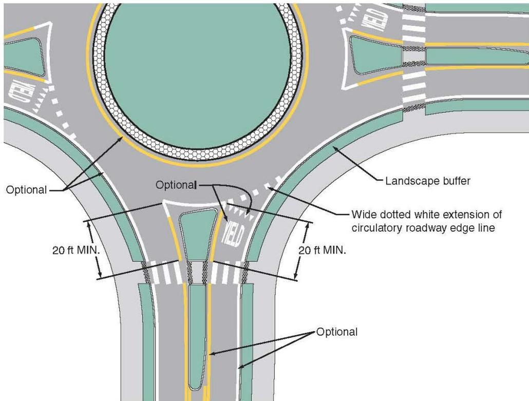
**Figure 3C-2. Lane-Use Arrow Pavement Marking Options for Roundabout Approaches**
