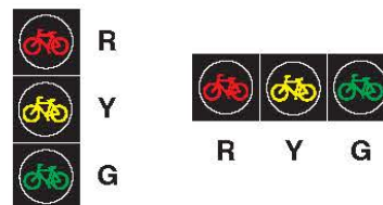
Figure 4H-1. Typical Arrangements of Bicycle Signal Faces
