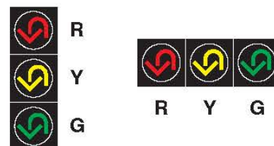
Figure 4E-1. Typical Arrangements of U-Turn Signal Faces
