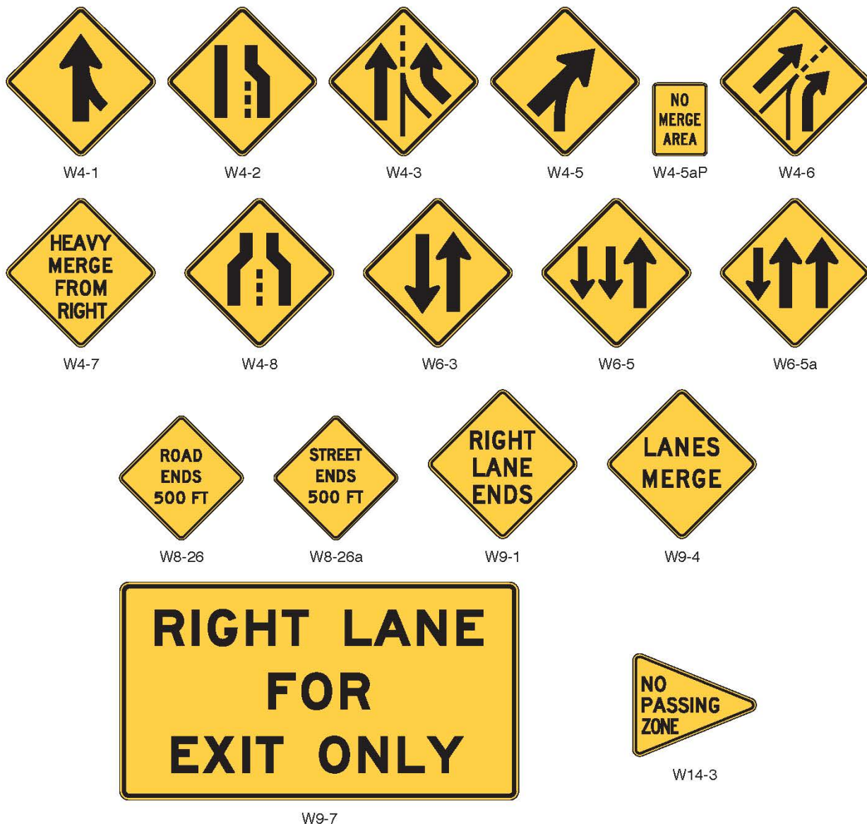
Figure 2C-11. Merging and Passing Signs and Plaques
