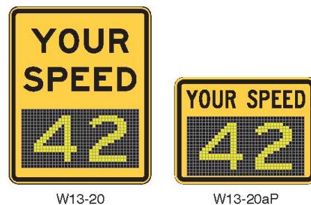
Figure 2C-4. Vehicle Speed Feedback Sign and Plaque
