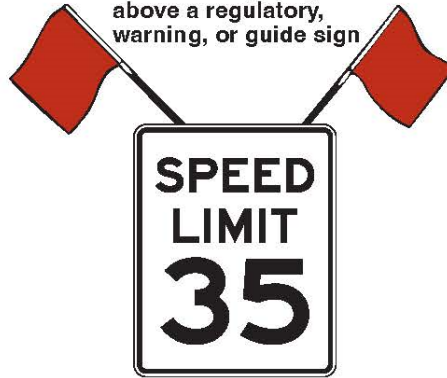
Figure 2A-1. Examples of Enhanced Conspicuity for Signs
