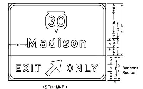
\* Minimum dimension is normally height of upper case letter. However the Exit Only Plaque may control the horizontal dimension of the sign. VERTICAL SPACING LAYOUTS
