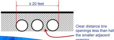
Clear distance b/w openings less than half the smaller adjacent opening
