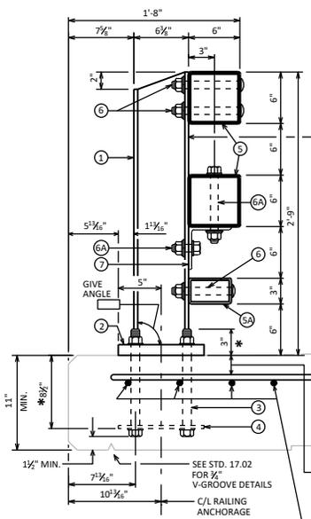
**SECTION THRU RAILING ON DECK**
