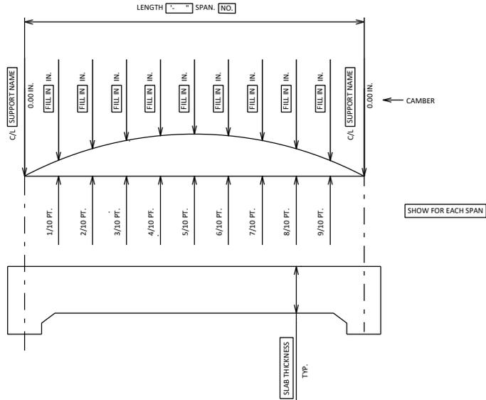
**CAMBER AND SLAB THICKNESS DIAGRAM**
