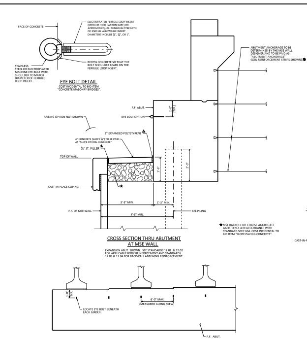
PARTIAL ELEVATION OF F.F. ABUTMENT SHOWING EYE BOLT FALL PROTECTION OPTION **DESIGNER NOTES**
