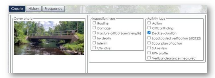
When just a portion of the deck is chained, do <u>not</u> select the Deck Evaluation activity. Document the results under the wearing surface element delamination defect 3210. Please include the specific area chained, the findings and the date chained.
