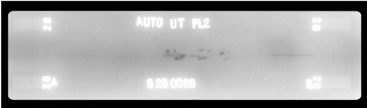
**Figure 5.9.1- 2:** RT image of weld. Note slag inclusions located in the center of the image and a lack of fusion located at right center.
