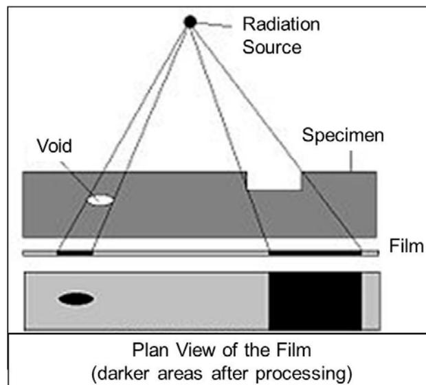
**Figure 5.9.1- 1:** RT of material with a void and notch. Note the darker areas on the film located below the test material.
