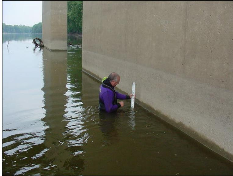
Figure 5.25.2.2-1: Inspector Using a Sounding Pole.
