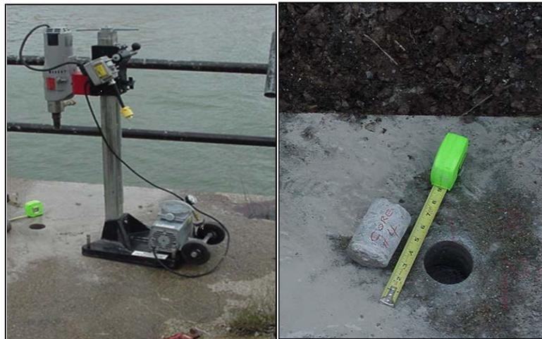
**Figure 5.23.4-1:** Concrete Coring Machine (Left) and Core Sample (Right).
