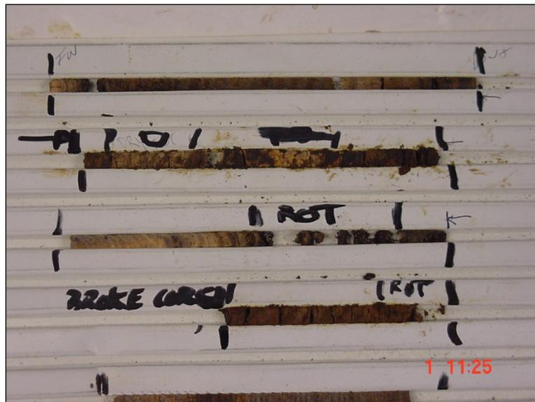
**Figure 5.23.6-1:** Typical Incremental Borer Core Samples.
