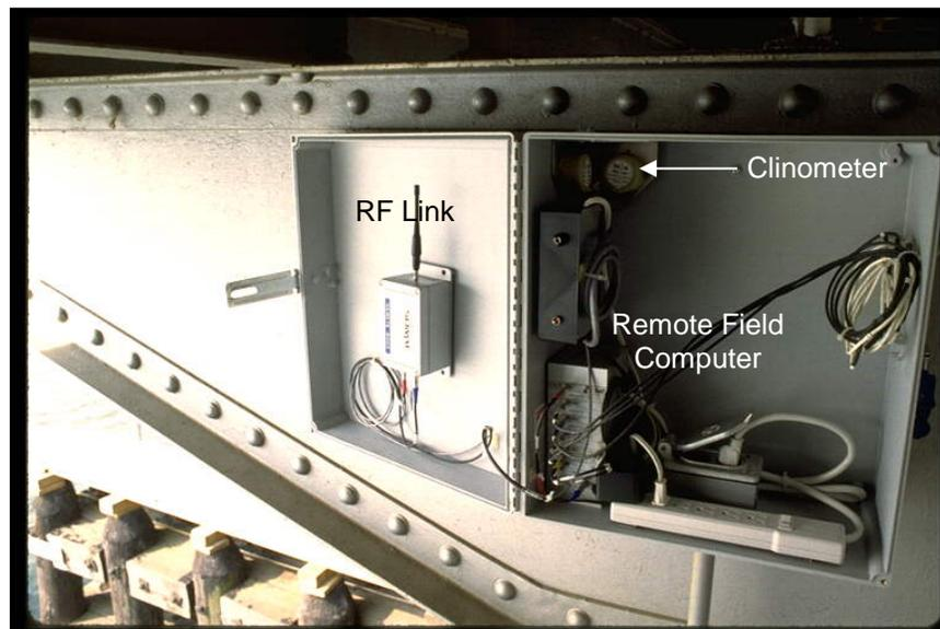
**Figure 5.22.1-1:** Remote Field Computer, Clinometers, and RF Link Mounted in Protective Enclosure.
