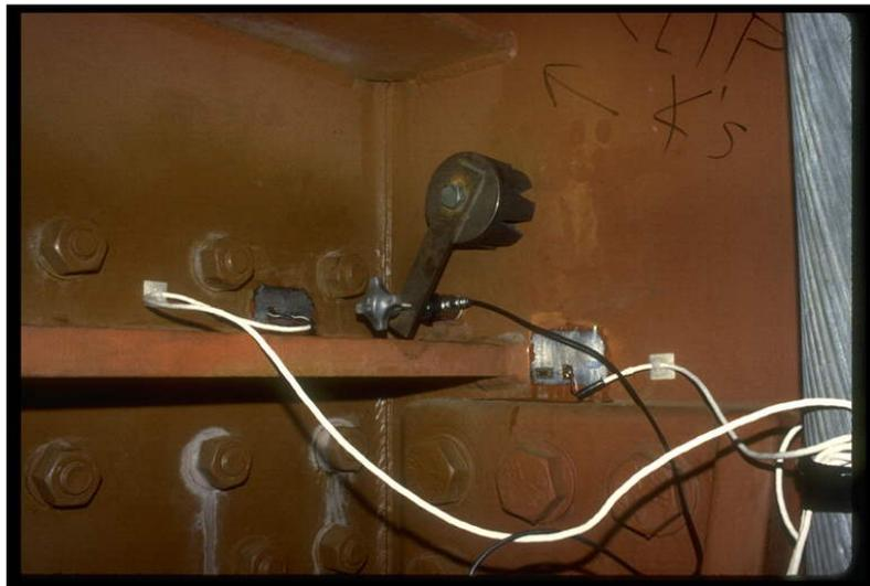
**Figure 5.22.1-3:** Strain Gauges Attached to the Tie Girders of a Tied Arch Bridge.
