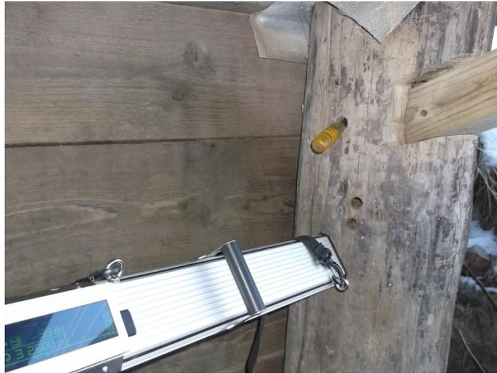
**Figure 5.20.2-1:** IML Resistograph, note the other old borings from a regular drill
