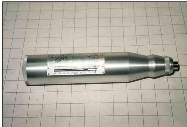
**Figure 5.18.1-1:** Standard Rebound Hammer.
