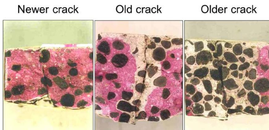
**Figure 5.17.1- 1:** Image of Cracked Concrete Samples After Carbonation Testing. Note the Older Crack and the Amount of Carbonation in the Concrete.
