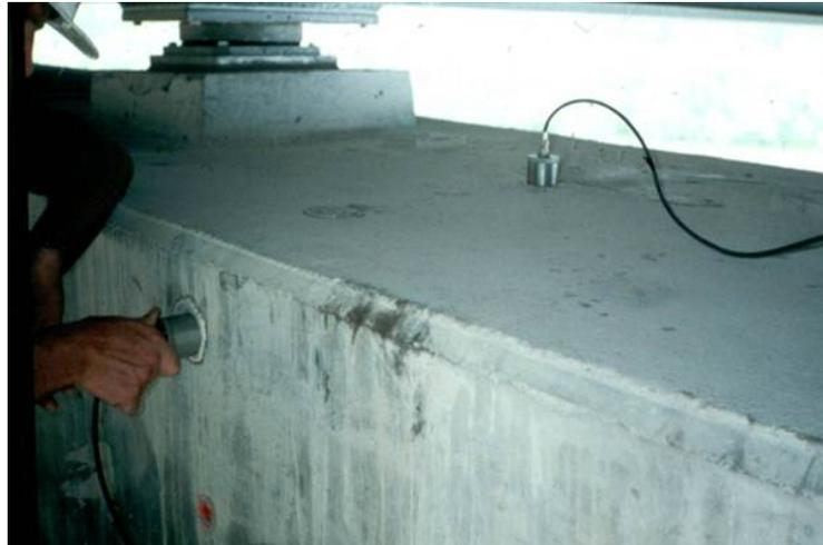
**Figure 5.13.2-1:** Inspector Conducting UPV on a Concrete Pier Cap Using Semi-Direct Transmission.
