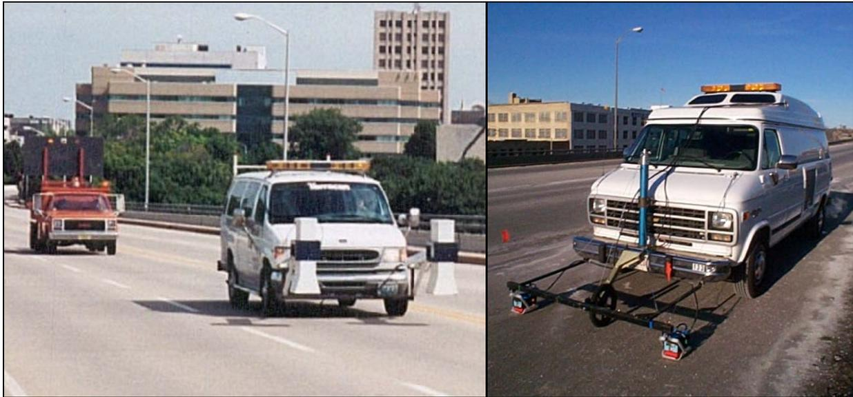
**Figure 5.10.1-2:** Horn Style (left) and Contact Style (right) Vehicle-Mounted Transducers.
