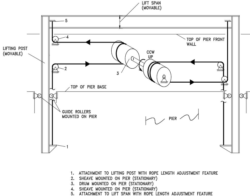
Figure 3.8.10.3-3: Stationary-Drum Equalizing System.
